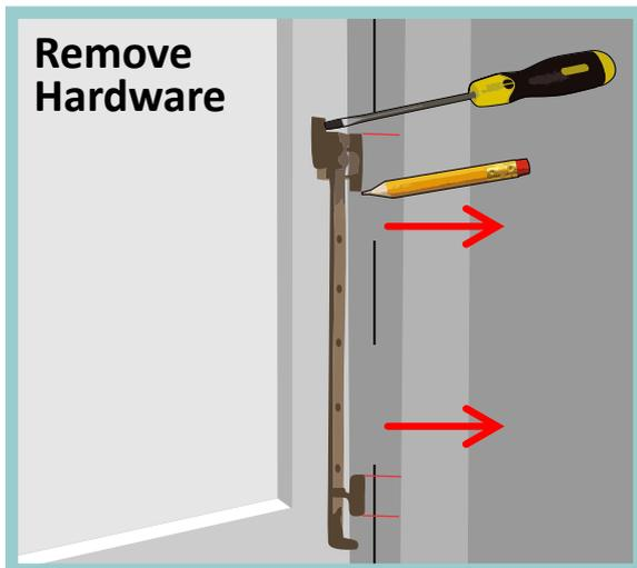
Remove existing window hardware so you can fit the new Draught Stop. The hardware will need to be refitted so mark out their height locations.
