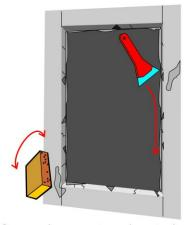
Check for rot by tapping the timber and listen for a dull thud. It may be repaired or need replacing
