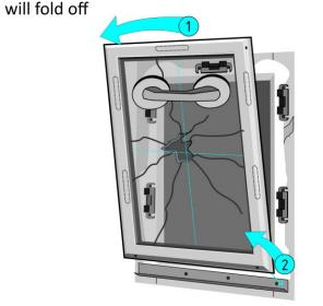
4/ Place the unit face down and remove the back profiles using the Pry bar from the inside edge
