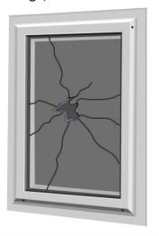
2/ Use a sharp knife and cut through the sealed edge. Place a suction cup as close to the top as possible
