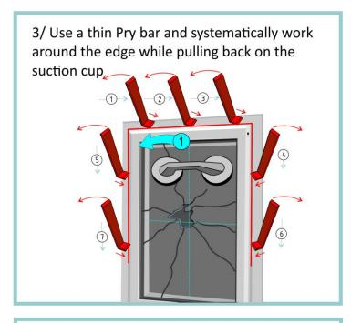
4/ The clip fixings will disengage and the panel
