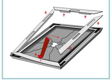
5/ The glass panel will be attached to the silicon edge seal so start at a corner and pull up the panel while holding down the edge profile
